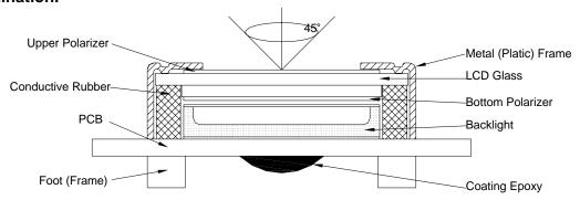
2. View Angle: with in 45° around perpendicular line.
